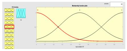
Fig. 2. Fuzzy sets with Gaussian membership functions of input variables  $x_i$ , i = 5, 6, 7, 8, 9
