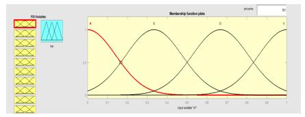
Fig. 1. Fuzzy sets with Gaussian membership functions of input variables  $x_i$ , i = 1, 2, 3, 4, 10
